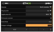
3. Navigate to the SBEC configuration tool and locate the [Output voltage] setting. Set the desired voltage output to complete the configuration.
