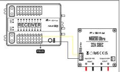
2. Ensure the receiver is connected to the SBEC via the S.Port/FBUS interface.
