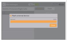
4. When the message changes to 'Flashing', wait for the progress bar to complete, this indicates that the firmware update is finished.
