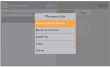
2. Copy the firmware file to the ETHOS radio. Use the File Manager tool to locate it, then select the file and choose "Flash external device."
