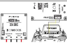
1. Disconnect the "+" wire, and connect only the "Signal" and "-" (Ground) wires from FBUS/S.Port port to the S.Port of your ETHOS radio.
