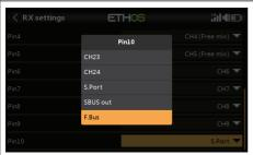
1. Bind the receiver with the radio, and set the port intended for SBEC connection to FBUS mode.
