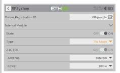
Then turn the state of Internal RF to On. Set the binding mode for the Internal RF module corresponding to the receiver (ACCST D16, ACCESS 2.4G, R9 ACCESS, TW,TD).
