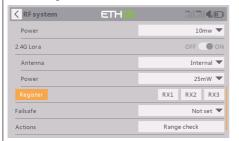
For TW Mode as an example, select the Set [Register] for getting the radio into Registration status in the RF System-Internal Module tool, then press the button on the receiver and power the receiver on.
