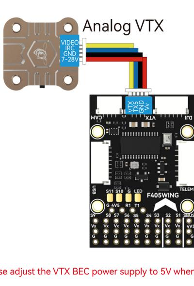
Note: Please adjust the VTX BEC power supply to 5V when using the TX800.
