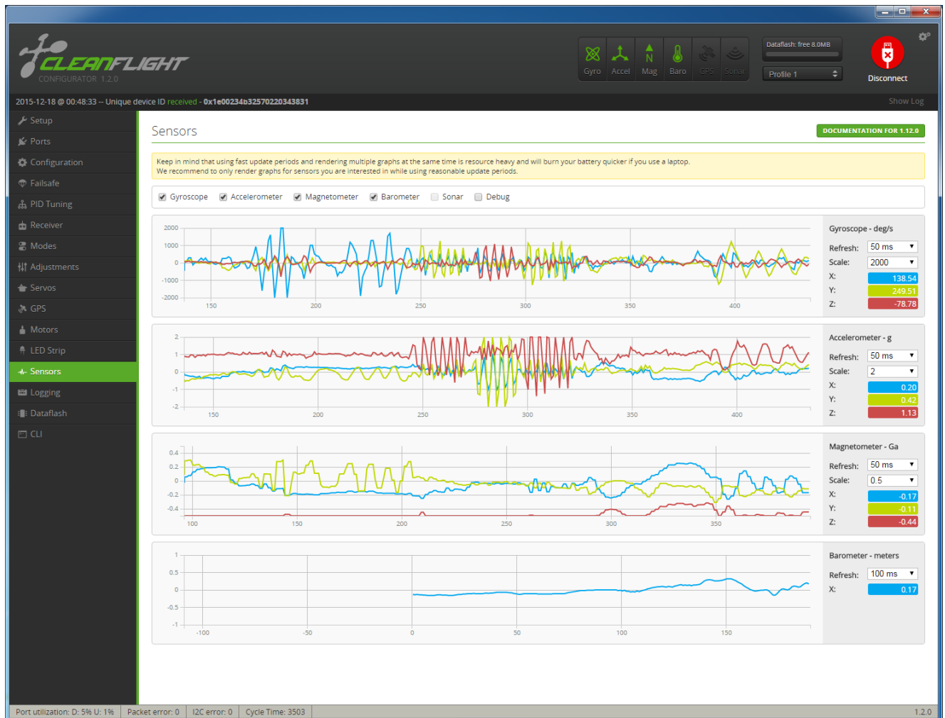
[Figure 4 - Sensors tab showing all sensors. Note: Only deluxe version has Mag and Baro]
