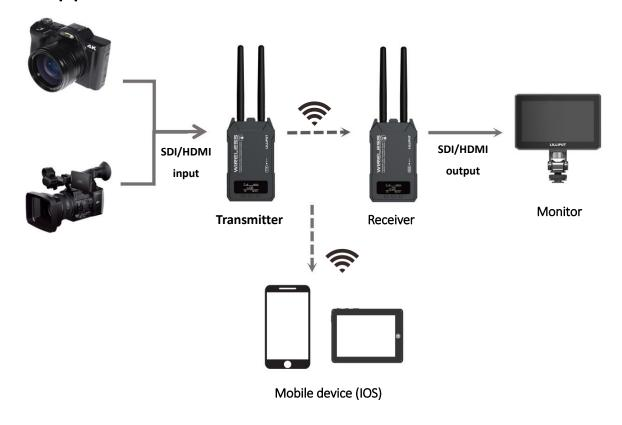
The connection process is shown in the diagram above. The camera and transmitter can be connected via an SDI/HDMI cable. After receiving video signal, the receiver outputs to monitor side via the SDI/HDMI cable.
