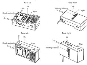
MSR66A should be mounted on the platform inside the airframe by using one of the
