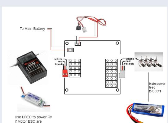
The completed Receiver and Motor wiring (for a QUAD Copter) looks like this:
