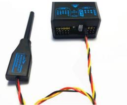
(2) Wiring method of airspeed meter and Arkbird Autopilot system OSDV3.1028 (autopilot 1.0), Please see picture as bellow: (After update Autopilot System with OSD to latest firmware V3.1028, it can be compatible with our airspeed meter.)
