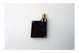
Remove the heat-transfer paste from the back of the video transmitter. Do NOT use any water to remove the paste.
