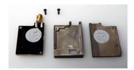
Open up the TBS UNIFY video transmitter and remove the aluminum case. Please try to avoid electrostatic discharge when handling the PCB.
