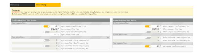
Correct filters will allow for higher PID's, and result in a more locked in feel.
