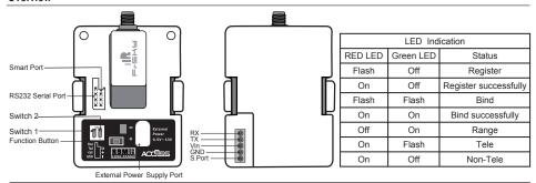
\* If the module is connected to both an external power and a transmitter, it will automatically be powered by the one with highervoltage.
