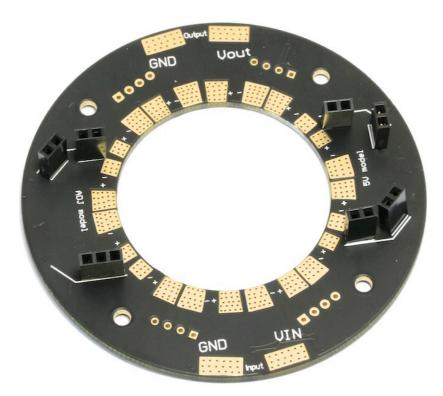
2. Next spilt the male header pins into  $6 \times 2pin$  and  $1 \times 3pin$  and then insert them into the pin connectors. Finally solder the UBECs onto the protruding pins – note that the adjustable UBEC sits on the left side and the  $5 \times 1pc$  UBEC on the right side.
