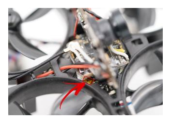
The bind procedure can take a couple of seconds. When the binding procedure is completed, the imperial march will stop playing. Power cycle both and ensure that the LED lights up green to signal a successful bind.
