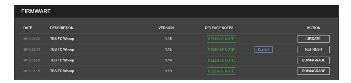
CURRENT indicates your current flight controller version. If there are more recent versions we recommend upgrading. Press UPDATE next to the most recent firmware revision on the top to switch to the newest firmware. Click UPDATE on the bottom of the next screen and wait a about 30 seconds for the update to complete. During this time the USB device will disconnect and reconnect once.
