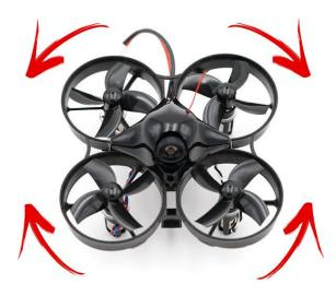
The propellers have clockwise and counterclockwise pitch angle. This means that one type of propeller will only generate adequate thrust for flight when spun in one direction. Here is how you identify the correct propeller for the motor directions:
