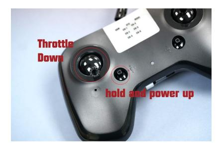
Power up your drone while holding the bind button. Use non-conductive materials (e.g. a toothpick) to push the bind button, and if necessary ask someone to help you as it usually requires three hands and not everyone has that many!
