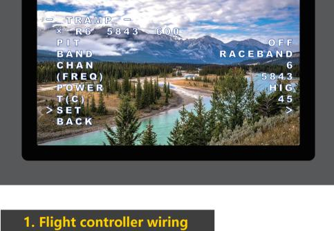
you need upload a VTX Table to the flight controller before using the remote control to modify the video transmitter parameters normally.
