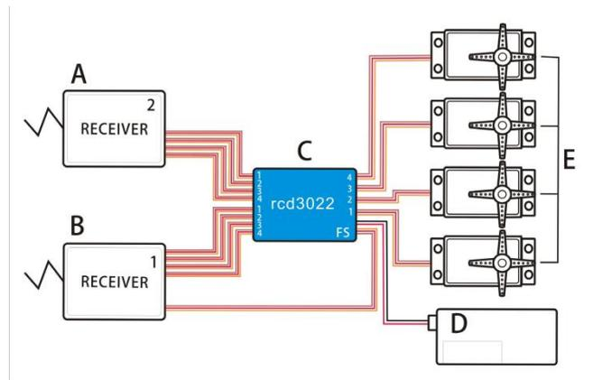
According to the above diagram, connect the receivers and servos with RCD3022, pay attention to connect them according to each number, FS signal should connect the prearranged port of the receiver, signal redundant function can be achieved by setting FS signal through the switch channel of transmitter.
